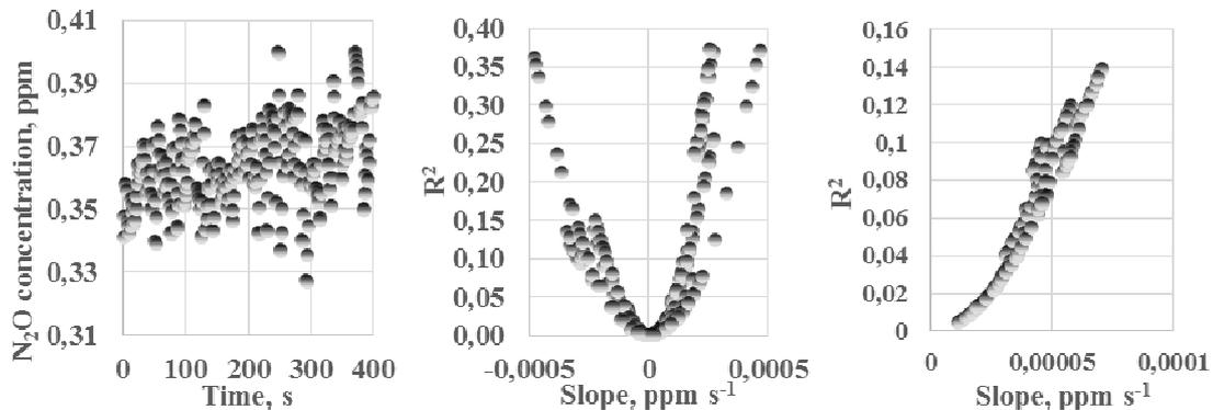
Fig. 5. Acceptable example of measurement (left-measured concentrations; middle –  $R^2$  and slope relation at 1minute calculation period; right –  $R^2$  and slope correlation at 4 minute calculation period)
