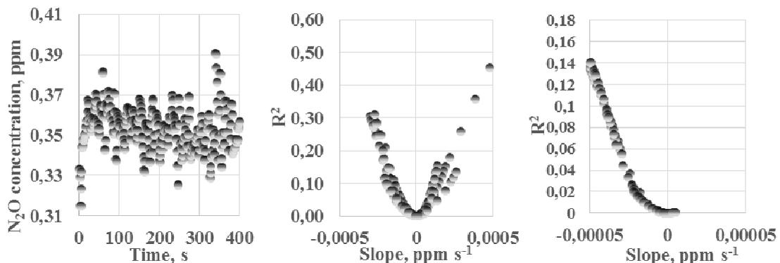
Fig. 6. Unacceptable example of measurement (left-measured concentrations; middle –  $R^2$  and slope correlation at 1minute calculation period; right –  $R^2$  and slope correlation at 4 minutes calculation period)
